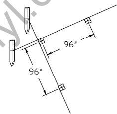
Important: The center to center measurement between any two posts should never exceed the center to center measurement of the fence style you purchase or your panels will not fit.
