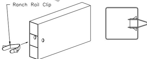
If using notches to secure your rails, notch both ends of the rail and secure the rail inside the post as shown in Figure 3.12.
